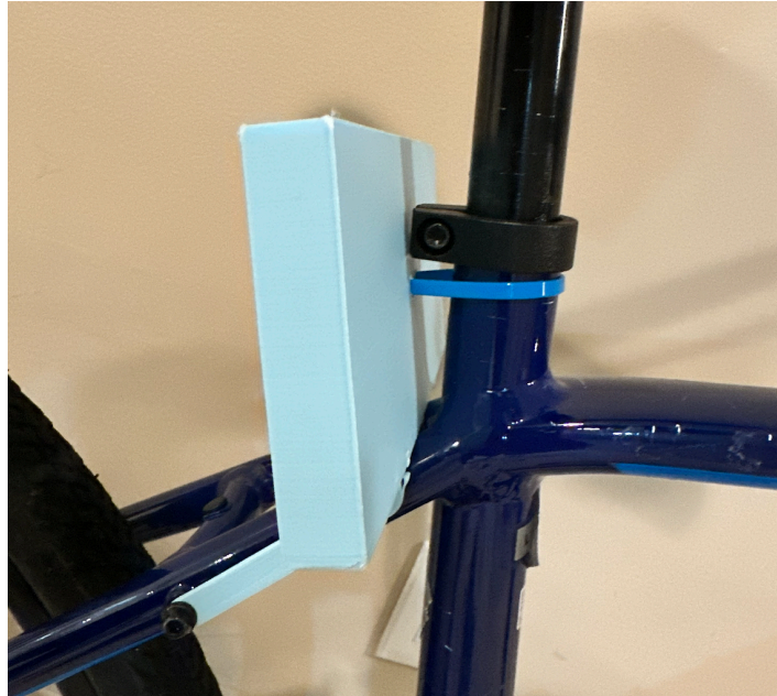
Figure 7.2.2: Zip Tie Around the Light Panel
